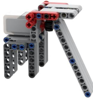
Press-mechanism to release the balls
